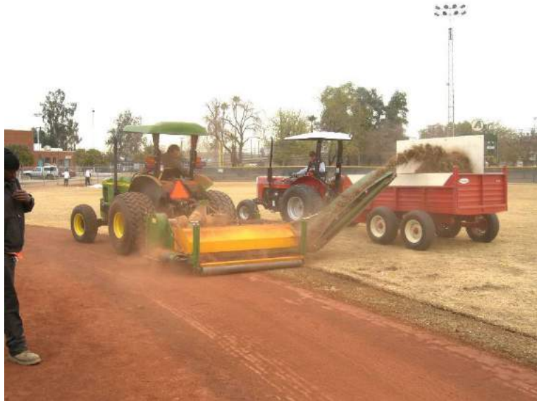
Top Maker Machine removing an infield lip in one pass
