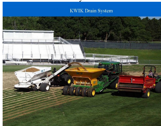
The KWIK Drain System, completely installed by equipment, can make tight clay soils percolate at 4" per hour the next day after installation.
