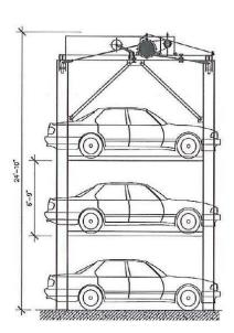
The diagram below provides a visual of the vertical height of the proposed stacker units, relative to surrounding elements, such as the garage and nearby residential properties.
