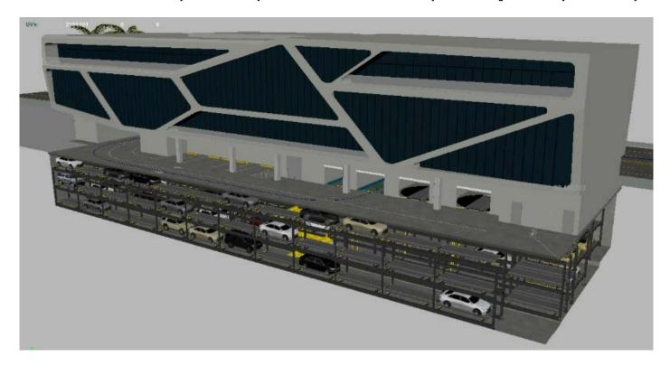
Since this parking structure is subterranean, there would be no visual impact on the surrounding properties. All movement happens within the enclosed bay and underground, therefore noise is not a factor. When standing 3' away from the bay, the decibel level of the lifts measures 65.
