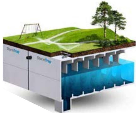
Figure 120. The SMQMP proposed several significant regional projects that include underground storage similar to what is shown in this concept diagram. Source: Culver City Stormwater Quality Master Plan, City of Culver City, 2021, page 110.
