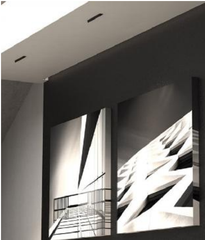
C Discreet, recessed, low glare adjustable downlights mounted at street side soffit and cantilevered ceiling at commercial entrance
