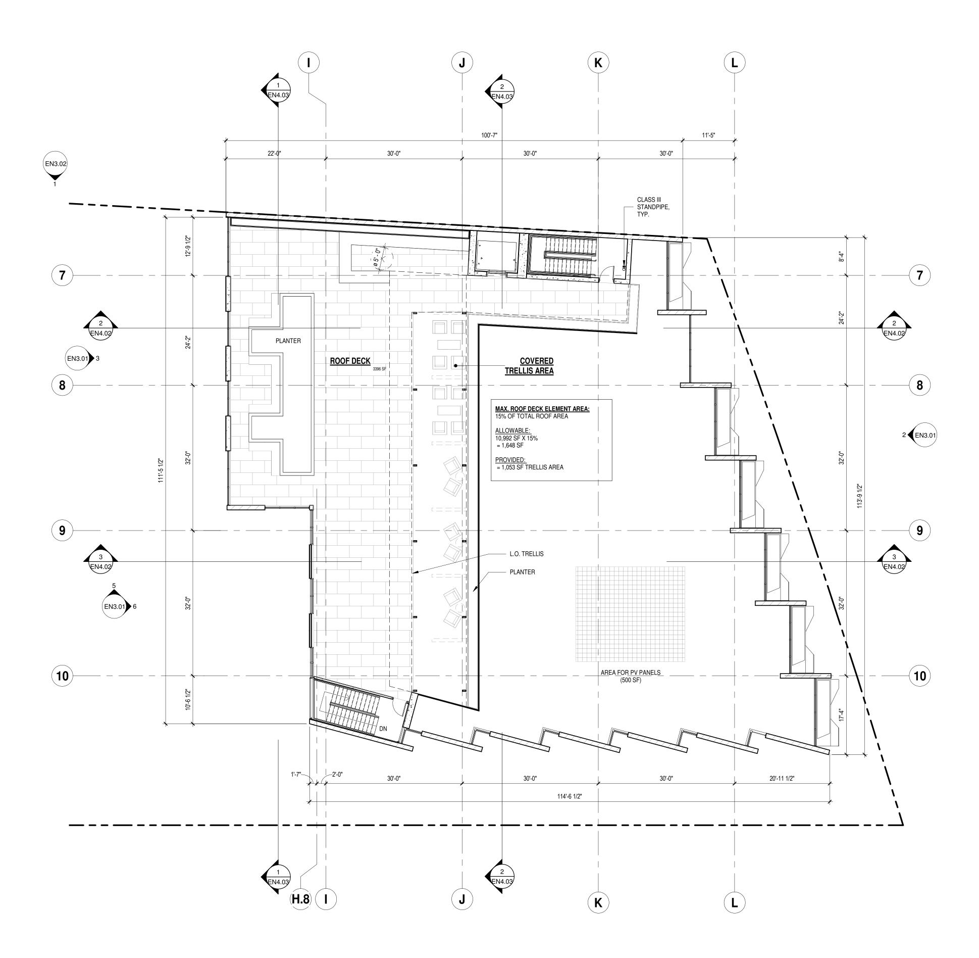
PLAN - NEW ROOF SCALE: 3/32" = 1'-0" ShubinDonaldson
