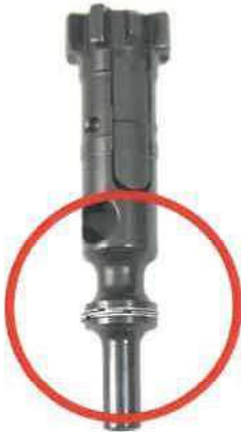
Correctly Staggered Gas Rings
