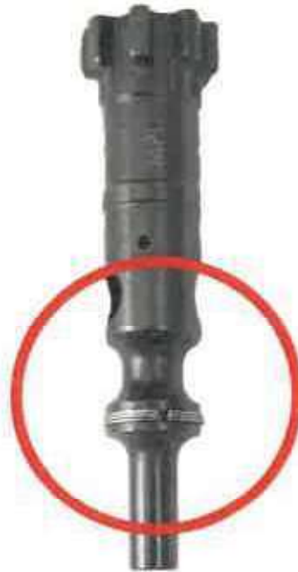
Incorrectly Staggered Gas Rings
