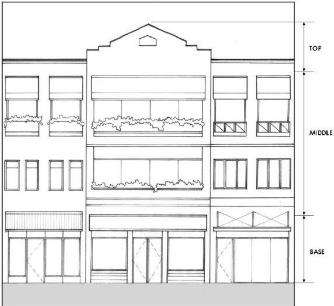
Figure 4-6 Building Elevation Composition
