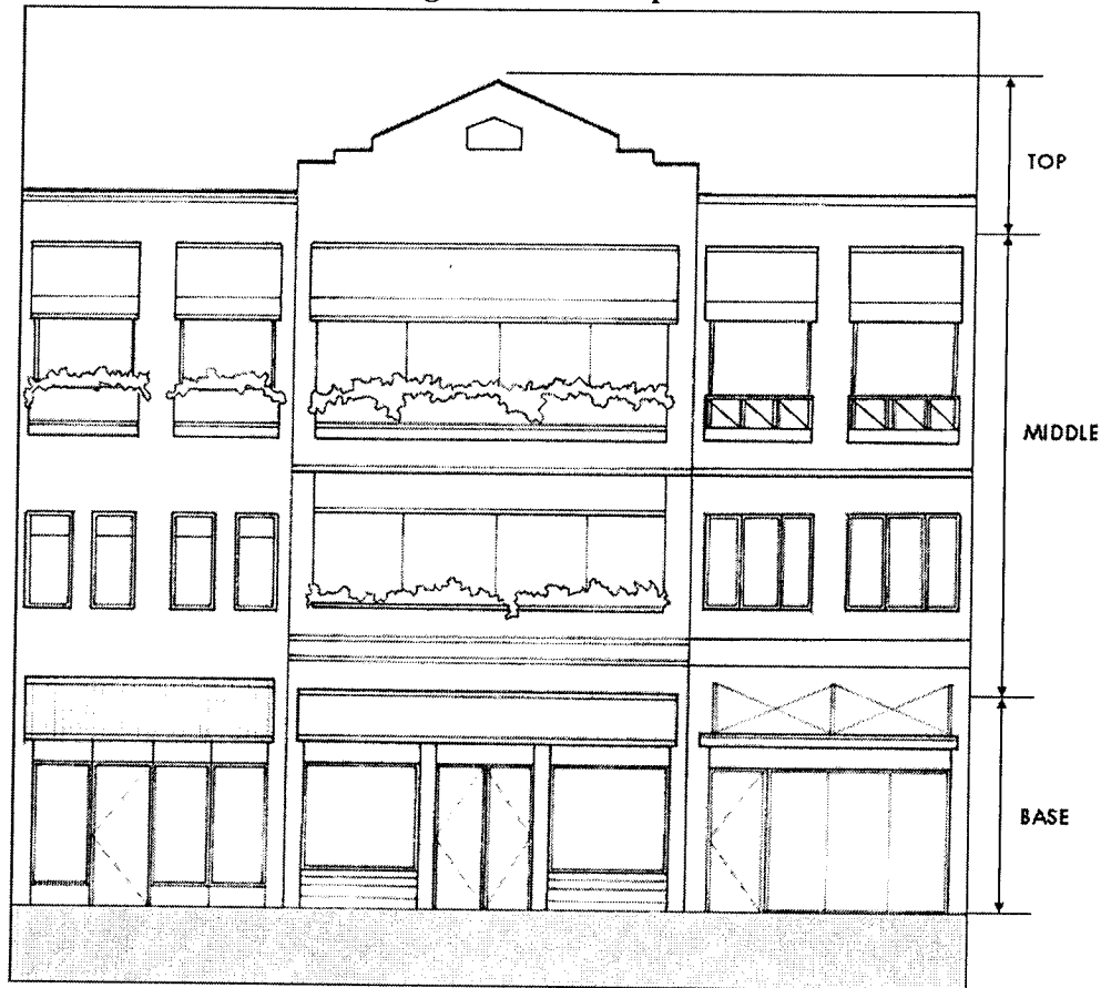
Figure 4-6 Building Elevation Composition
