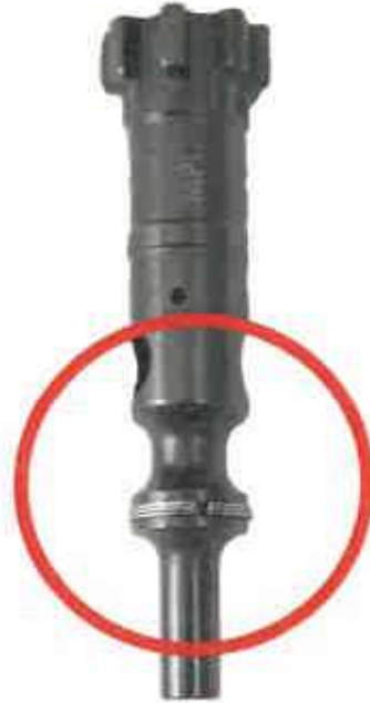
Incorrectly Staggered Gas Rings
