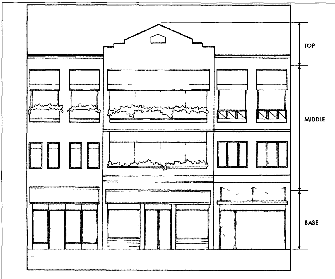
Figure 4-6 Building Elevation Composition
