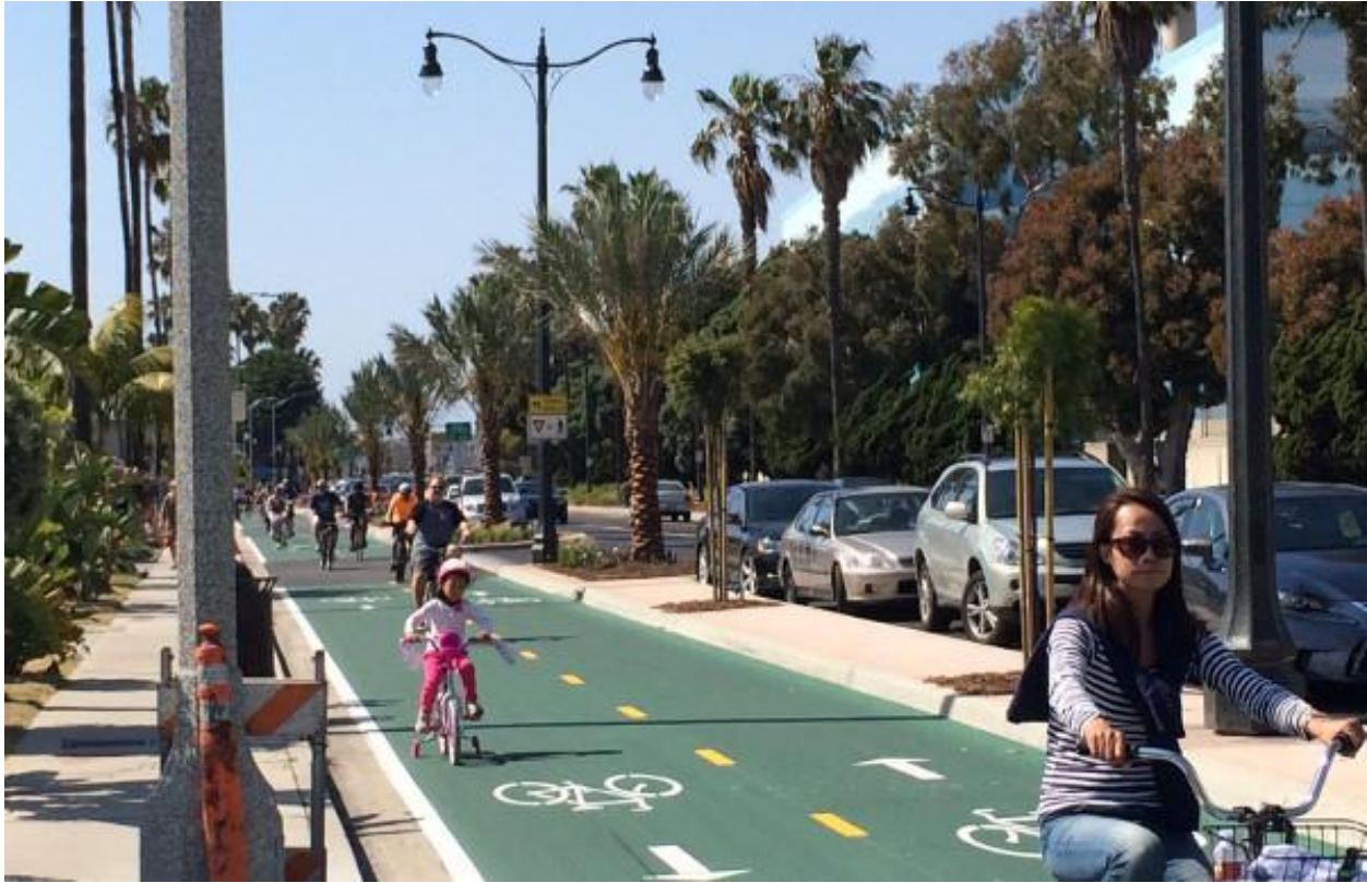
A two-way protected bike lane in Redondo Beach functions like a bike path on one side of the street. Photo: Rock Miller
