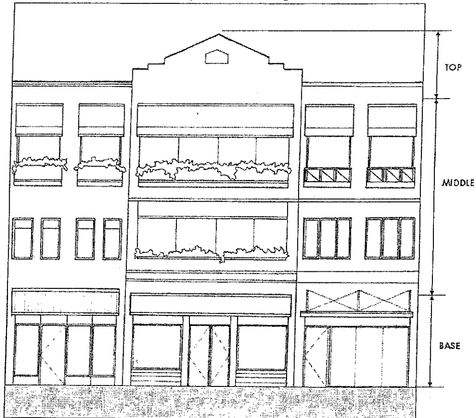
Figure 4-6 Building Elevation Composition
