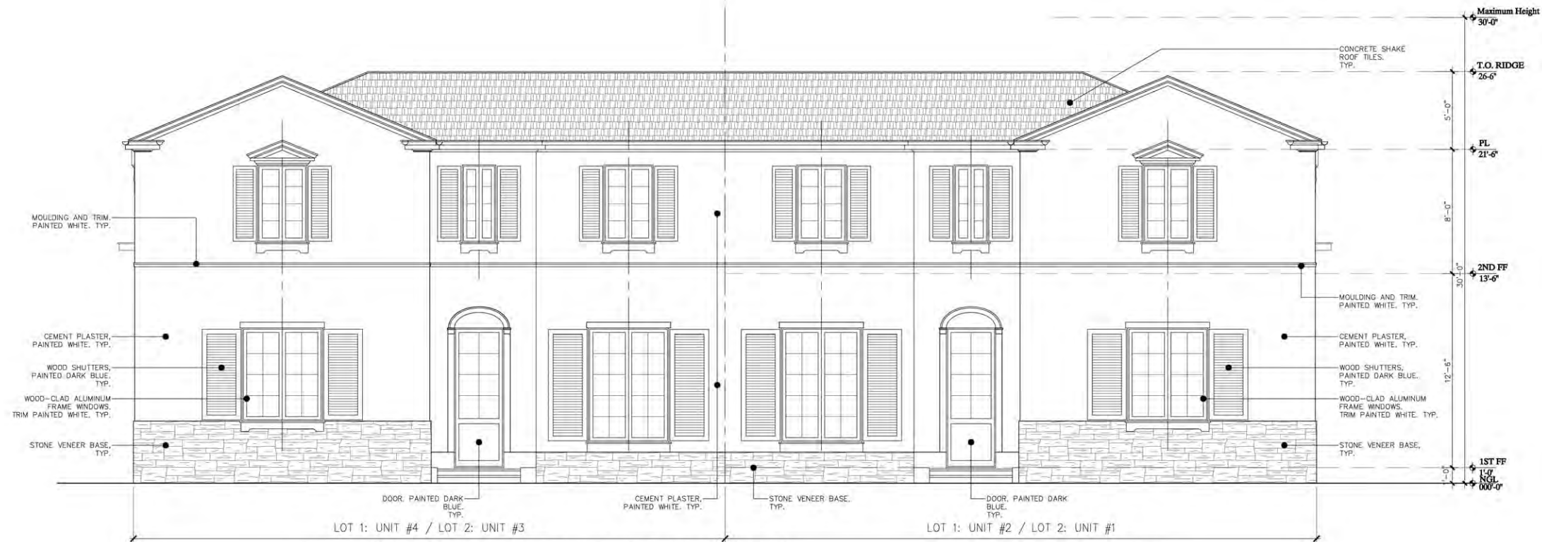
(INTERIOR) LOT 1: UNITS #2 & #4 SOUTH ELEVATION (INTERIOR) LOT 2: UNITS #1 & #3 NORTH ELEVATION (SAME, MIRRORED) SCALE: 1/4" = 1'-0"
