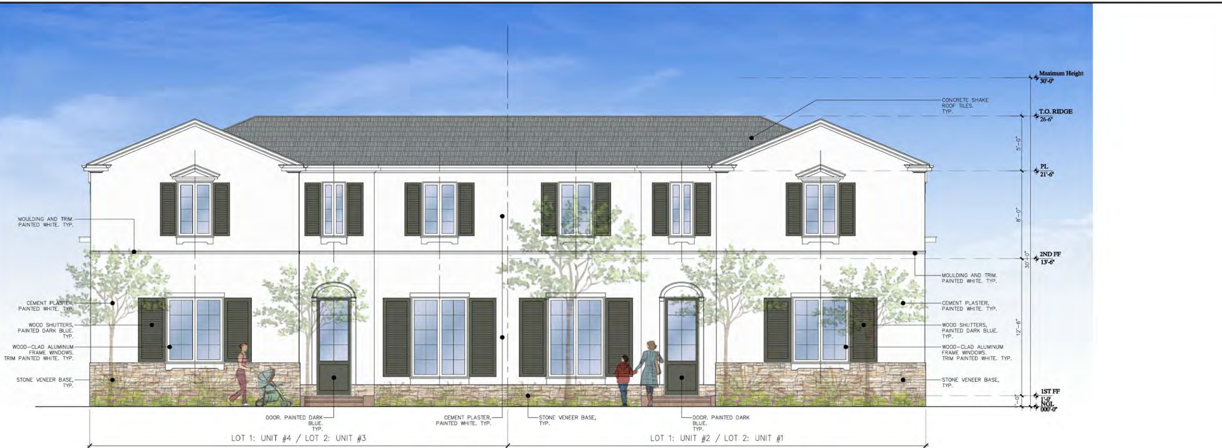
(INTERIOR) LOT 1: UNITS #2 & #4 SOUTH ELEVATION (INTERIOR) LOT 2: UNITS #1 & #3 NORTH ELEVATION (SAME, MIRRORED) SCALE: 1/4" = 1'-0"
