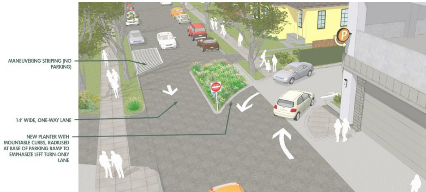
Figure 19 Alternative 1 - Colonial Traffic Calming Configuration
