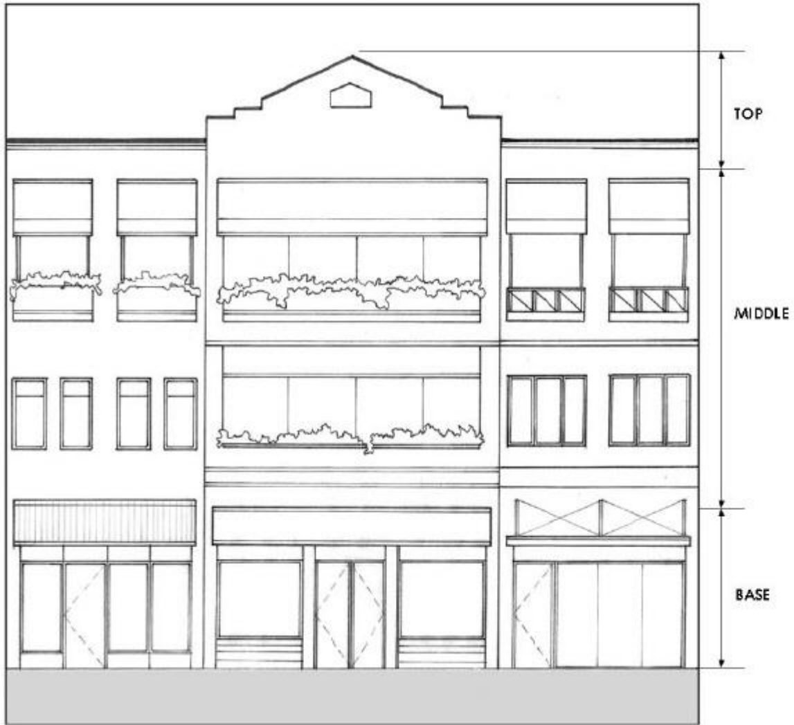
Figure 4-6 Building Elevation Composition
