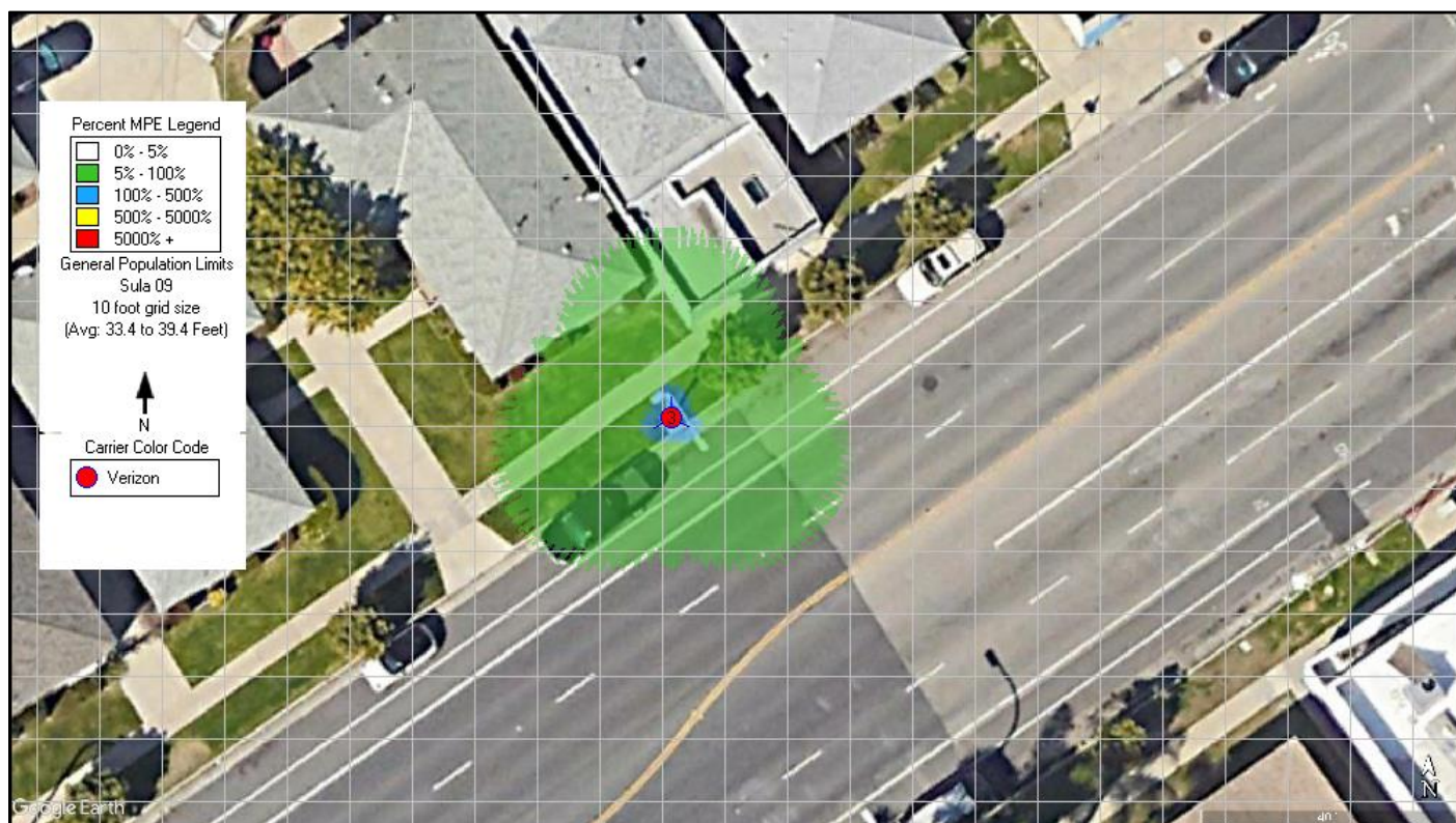
Figure 3: Top-Down View at Antenna Level MPE limits
