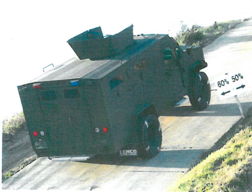
Figure 4. The BearCat ascending the 60-percent longitudinal grade.
