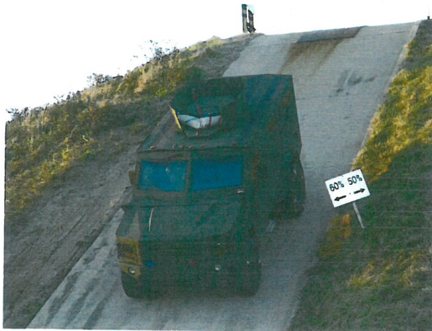
Figure 5. The BearCat descending the 60-percent longitudinal grade.
