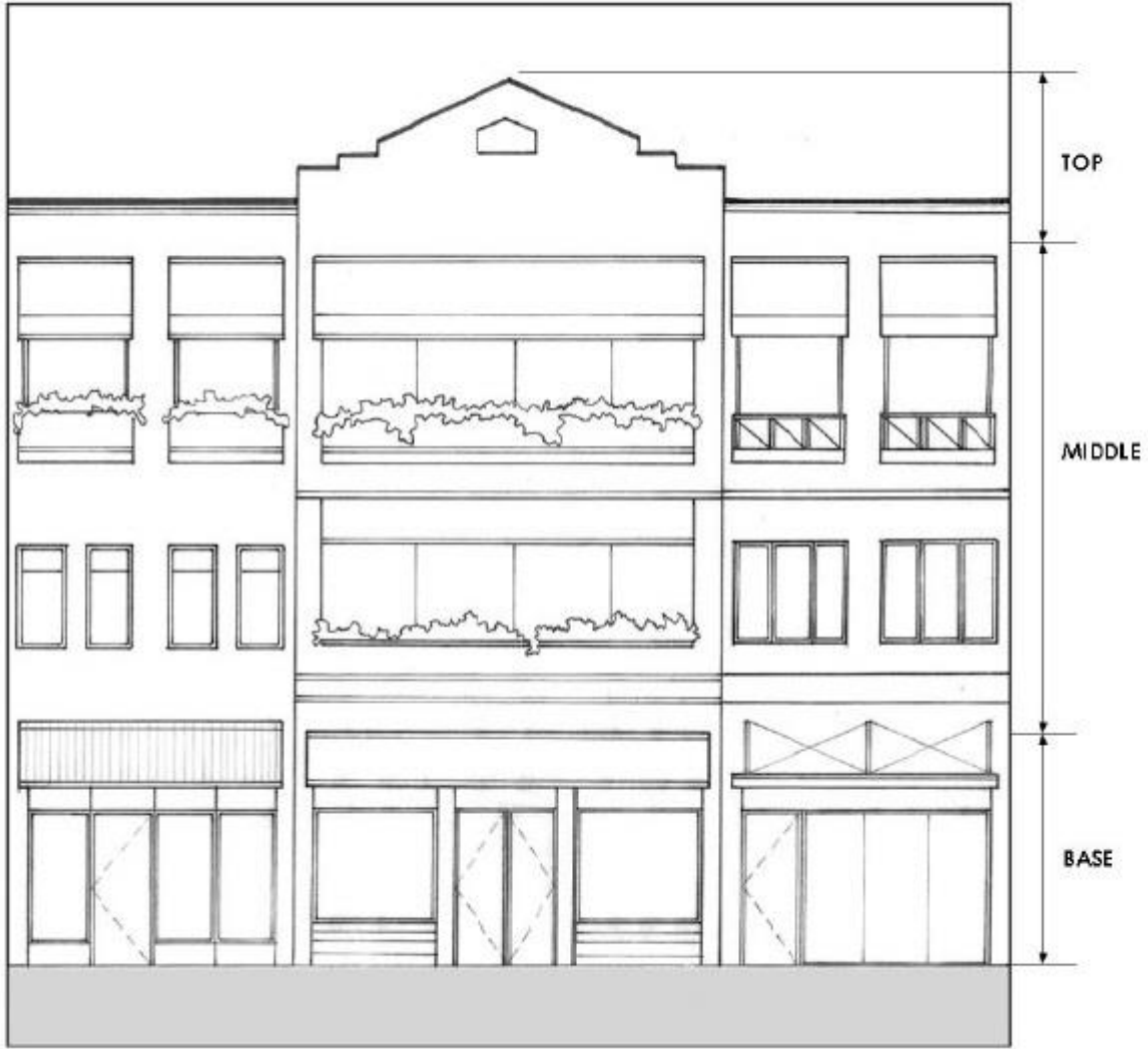
Figure 4-6 Building Elevation Composition
