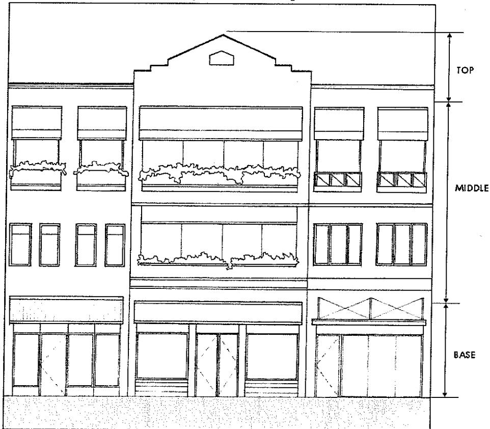
Figure 4-6 Building Elevation Composition
