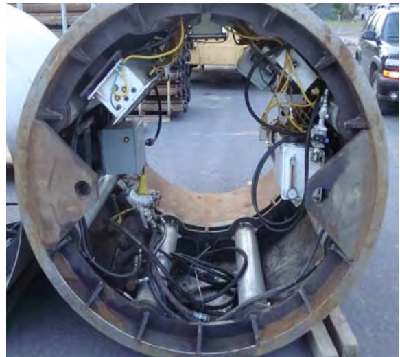
Recoverable Jacking Can with over 600 tons of thrust capacity
