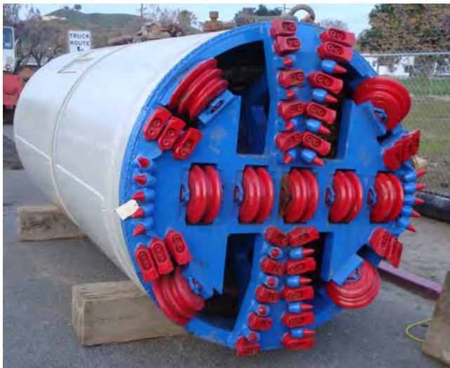
Akkerman Microtunneling Boring Machine (MTBM) and a mixed-ground cutterhead with a combination of Palmieri roller (disk) cutters and carbide teeth
