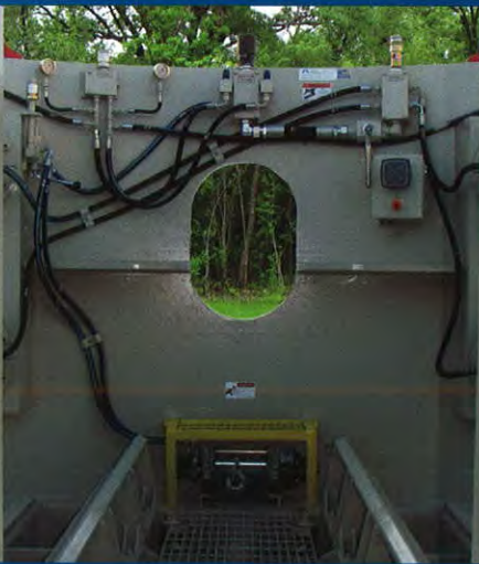
The laser guidance slot is visible here along with the frame's hydraulics and the winch pullback for the thrust block.
