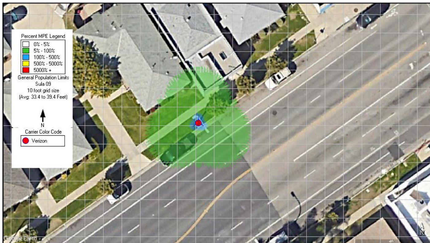
Figure 3: Top-Down View at Antenna Level MPE limits
