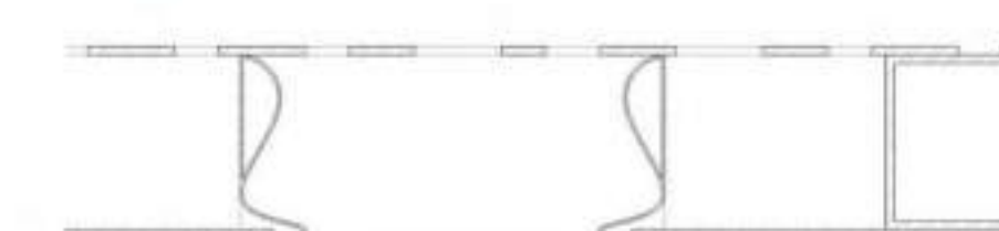
SLIDING PANEL HANDLE DETAIL
