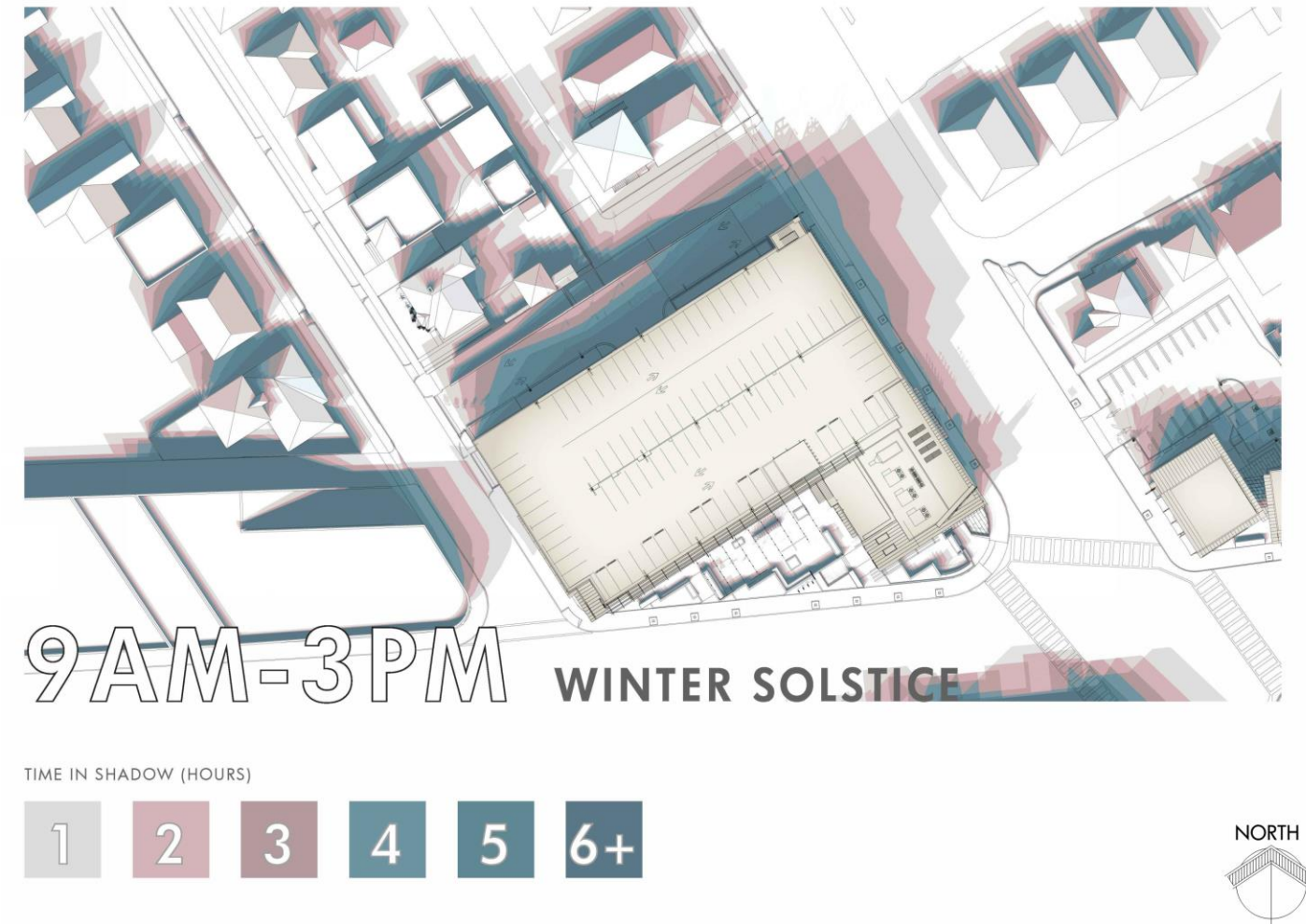
Figure 23 Site A - Enlarged Shade and Shadow Diagram
