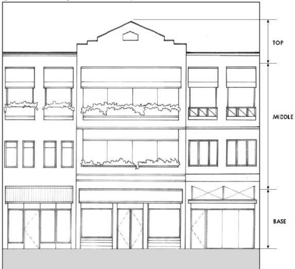
Figure 4-6 Building Elevation Composition
