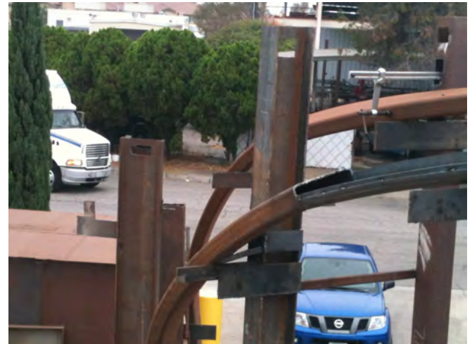
Fabrication photos of " re currents ": induction roll forming: bending and twisting Fabricator: Paramount Roll Forming
