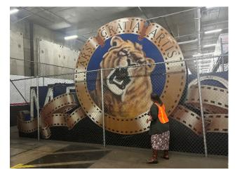
At the base, the curvature has been infilled with several sections of plywood cut to follow the arc of the logo on the upper edge and squared off at the bottom to sit flush with the floor. The purpose of this plywood intervention is unclear; it appears temporary, non-structural, and not load-bearing. The method of attachment between the painted sign faces and the internal bracing remains undetermined.
