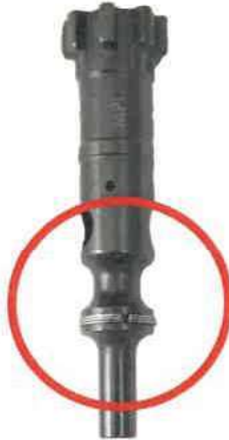
Incorrectly Staggered Gas Rings
