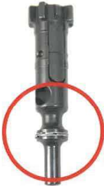
Correctly Staggered Gas Rings
