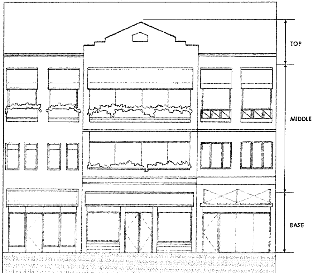
Figure 4-6 Building Elevation Composition
