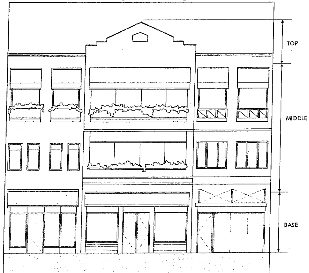
Figure 4-6 Building Elevation Composition
