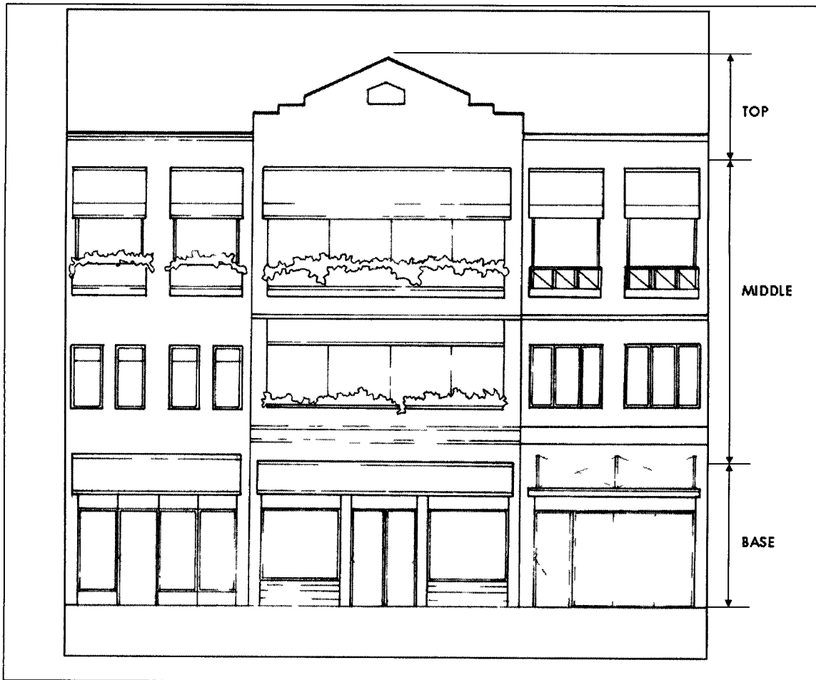
Figure 4-6 Building Elevation Composition
