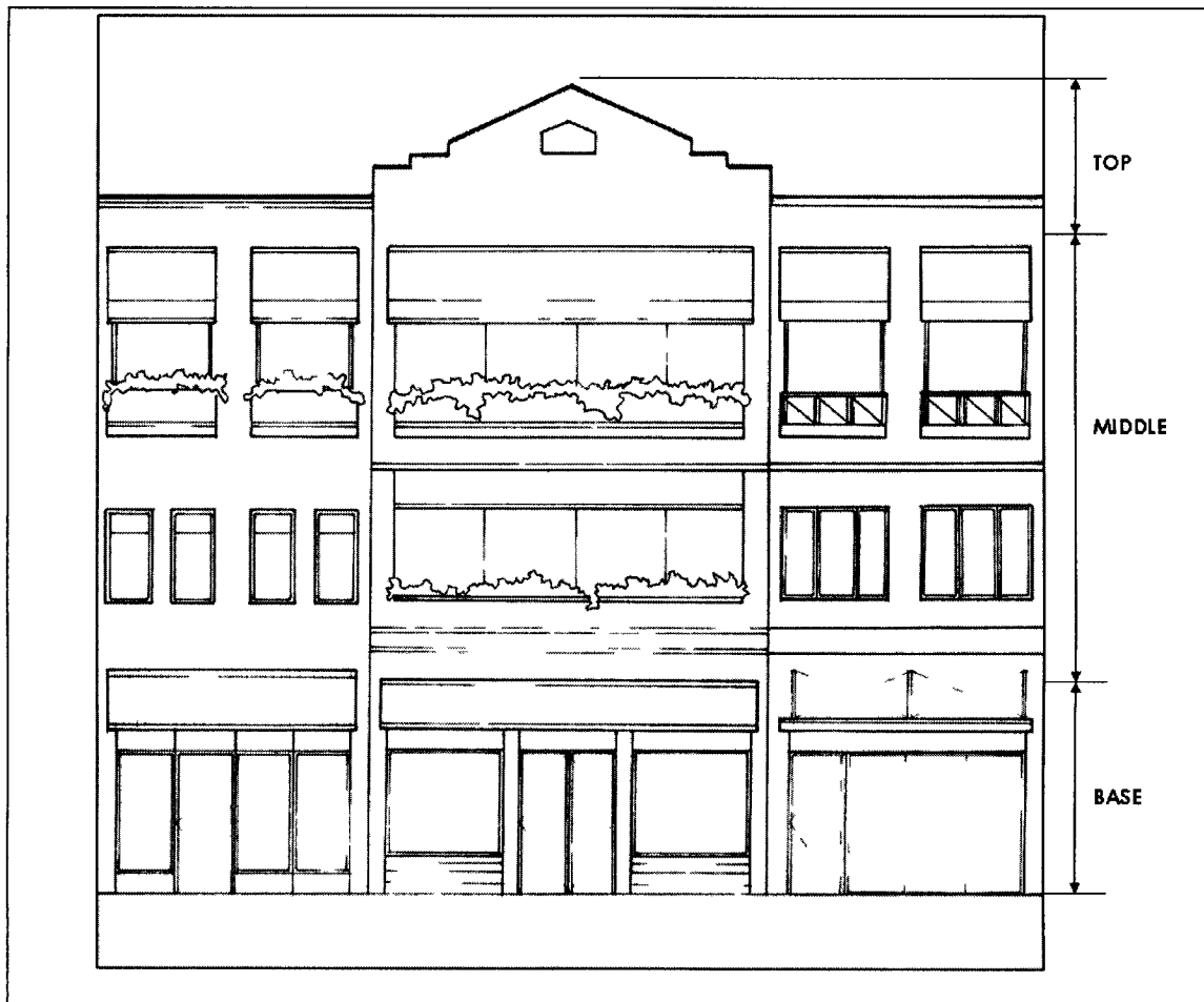
Figure 4-6 Building Elevation Composition
